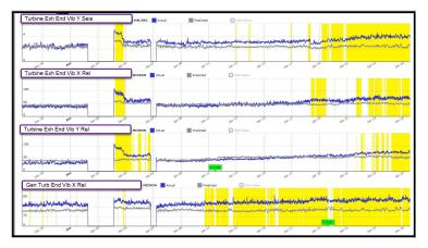
Gas turbine vibration changes identify developing bearing fault
