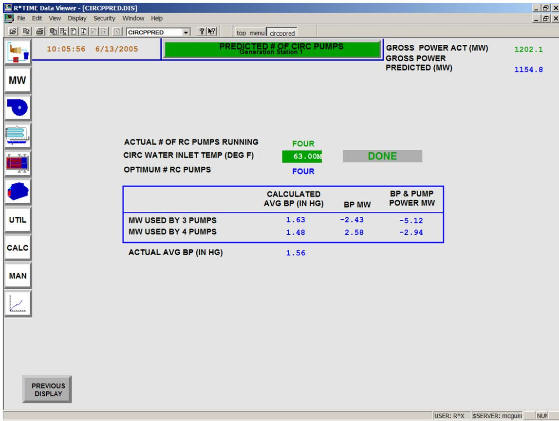
Figure 3: Sample Predictive Display for Circulating Pump Operation
