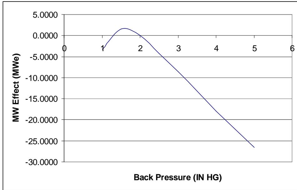
Figure 1: Example Back Pressure MW Effect Curve
